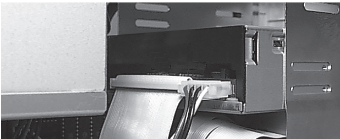
Installing Power Cable
